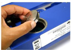
The SIM card is accessed via this waterproof cap located on the bottom of the module.
